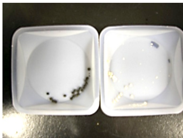
Fig. 2 Left: original black grains; Right: material out of the muffle furnace
